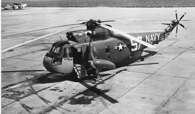
Prototype XHSS-2s passed their Navy trials at Patuxent River and set new helicopter speed records.
