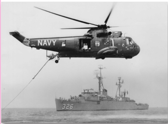
The RH-3A with towed cable cutting array gave the US Navy its first operational mine-sweeping helicopter.
