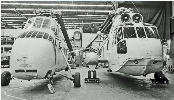
An S-58/HSS-1 and the S-61/HSS-2 mockup provided a dramatic size comparison in 1958.
