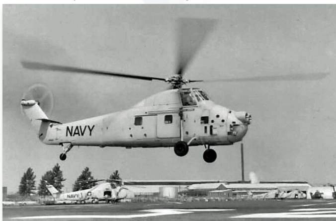
Sikorsky modified two S-58s to HSS-1Fs. Twin T58 turboshafts replaced a single Wright radial piston engine.
