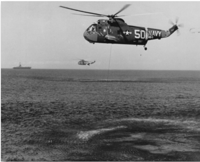
The Sea King automated the sonar-dipping hover for anti-submarine warfare at night and in adverse weather.
