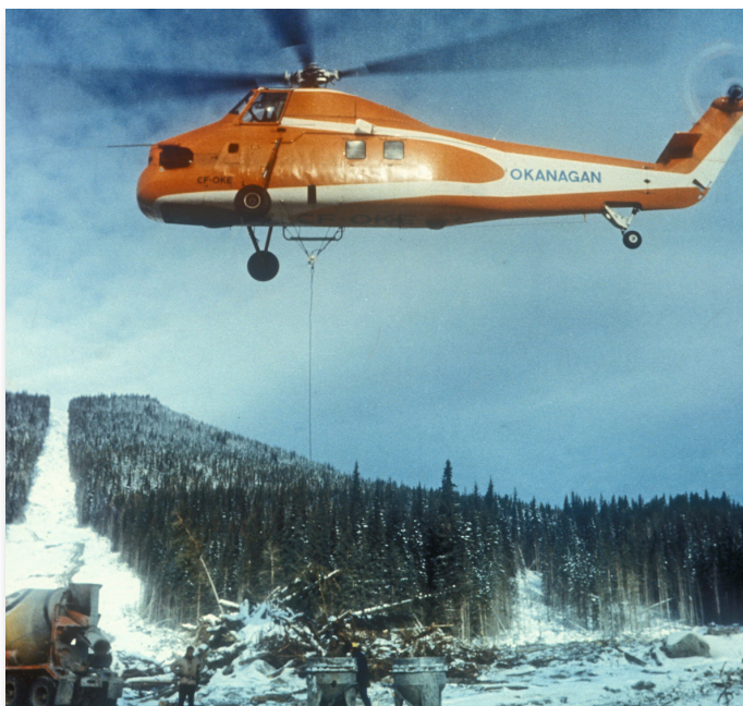
Canadian operator Okanagan Helicopters converted several S-58Bs to turbine S-58Ts.
