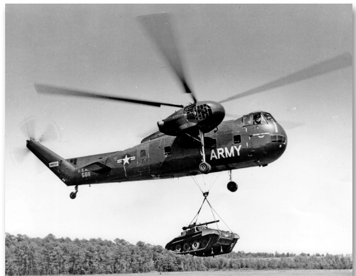
The Army CH-37A carried heavy external loads such as the M50 tracked vehicle.
