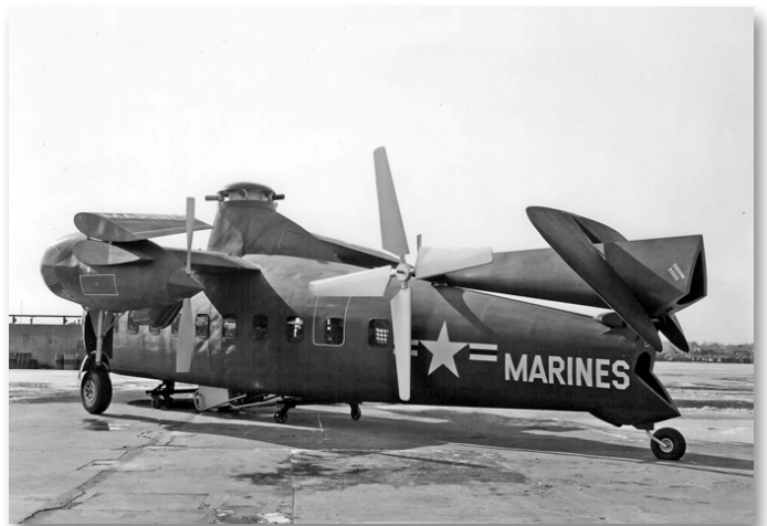
The S-56B mockup showed a compound helicopter with folding wings and pusher props.
