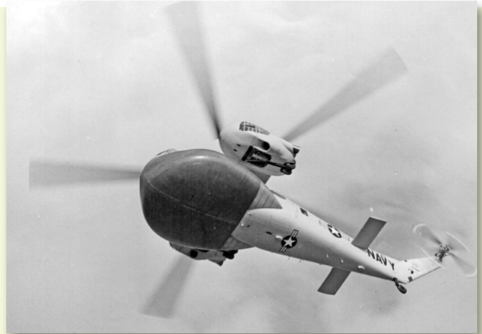
The Navy tested the HRS2S-1W with a large radome for airborne early warning.
