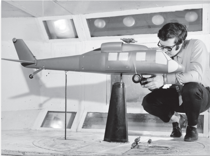
Sikorsky engineers tested the S-70 configuration in the United Technologies wind tunnel.
