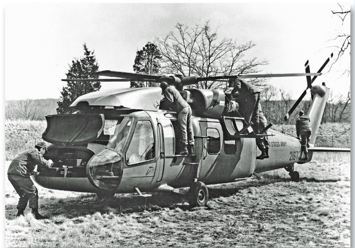
The UTTAS wood mockup showed the integrated workstands and other features of the YUH-60A.
