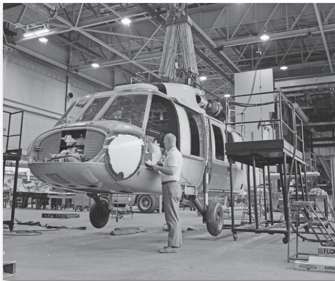
The Static Test Article was subjected to wide-spectrum vibration to measure YUH-60A airframe response.
