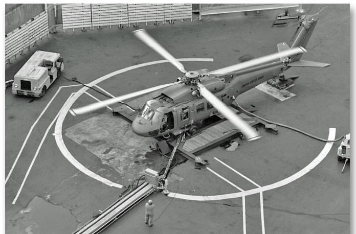
The Ground Test Article proved the reliability of the YUH-60A drivetrain.
