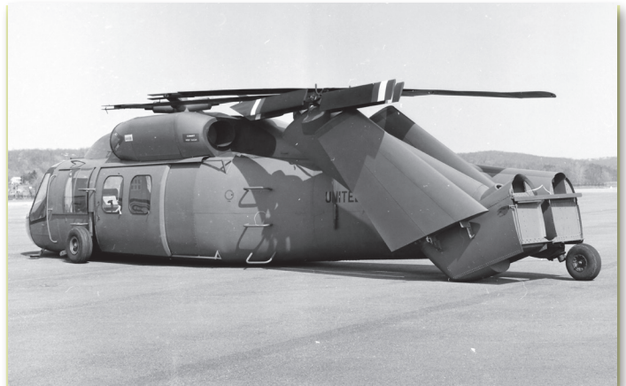
The folded mockup demonstrated YUH-60A air transportability features.
