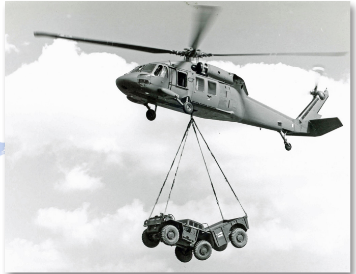
The YUH-60A with full fuel lifted the Gama Goat vehicle during Government Competitive Testing.
