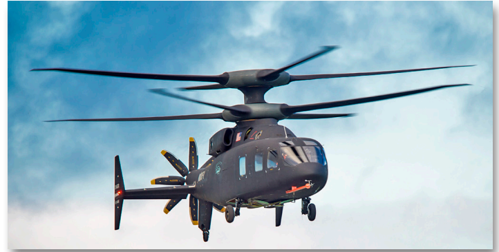
The SB>1 Defiant Joint Multi Role Technology Demonstrator achieved 247 kt with X2 technologies.
