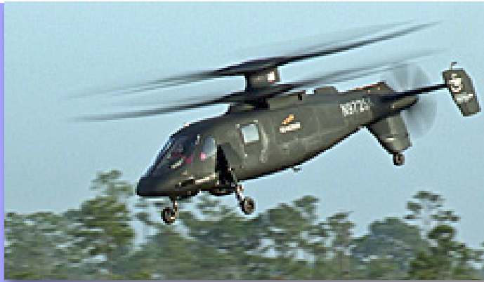
The S-97 with integrated auxiliary propulsion demonstrated 200 kt speed and tactical agility.
