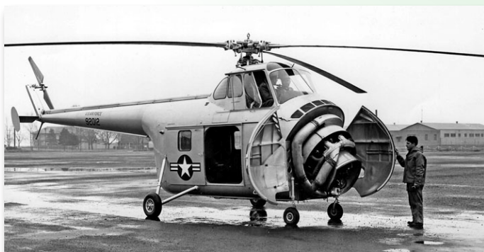
The company-funded S-55/YH-19 put the engine up front to remedy cg limitations.
