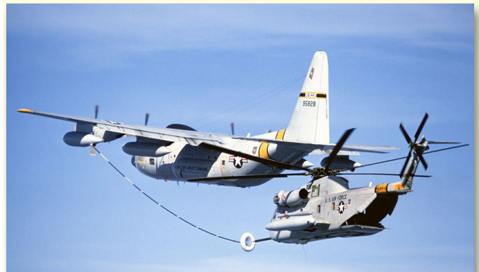
The HH-53C, here refueling from a Hercules tanker, further extended the reach of rescue squadrons. (US DoD)
