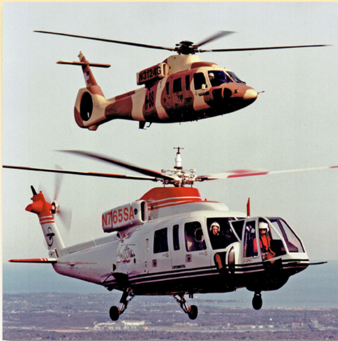
The S-76 Fantail and Shadow flew technologies key to the RAH-66 Comanche.
