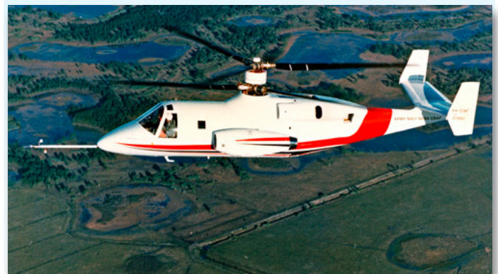
At the DFC, the S-69 (XH-59) attained 263 kt and introduced the Advancing Blade Concept. (NASA via DVIDS)
