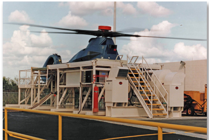
The RAH-66 Propulsion System Testbed tested the drivetrain of the stealthy scout before first flight.
