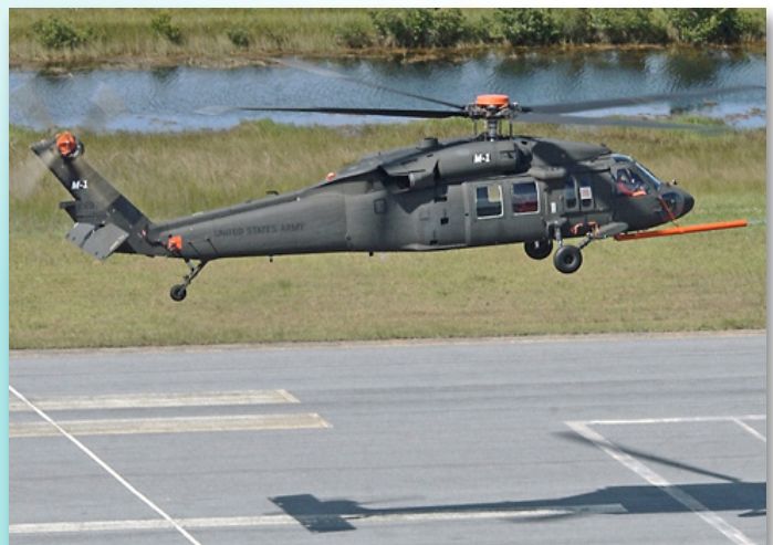
The first UH-60M flown at West Palm Beach in 2003 was a recapitalized UH-60A.
