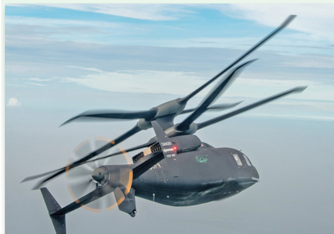
The S-100 (SB>1) Joint Multi Role Technology Demonstrator assembled at the DFC applied X2 technologies to the Army Future Vertical Lift Initiative.
