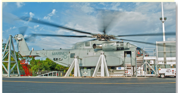
The CH-53K ground test vehicle at West Palm Beach tested the heavy lift helicopter drivetrain and structures.
