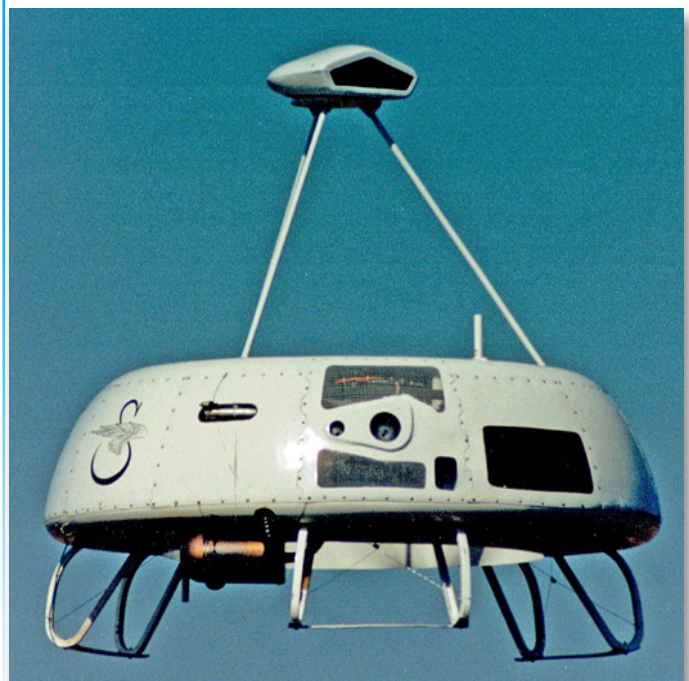
The Cypher Unmanned Air Vehicle used Comanche ducted fan technology.
