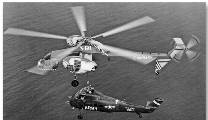
The company-funded S-60 demonstrated the potential of the crane helicopter, here carrying an Army H-34.
