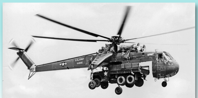
The S-64 (Army CH-54 Tarhe) gave the Army a Skycrane with turboshaft power to lift heavy external loads.
