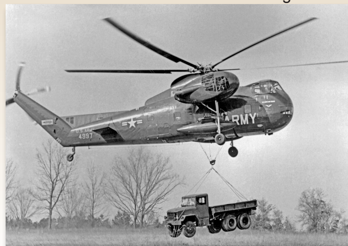
The twin-engine S-56 (Army H-37 Mojave) was a “medium” cargo helicopter with cabin space for 26 troops and power to carry heavy cargo.
