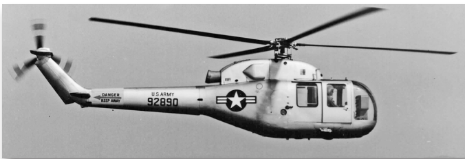
Modified from the S-52 (Army XH-18), the fast S-59 (Army XH-39) was Sikorsky's first turbine-engined helicopter.
