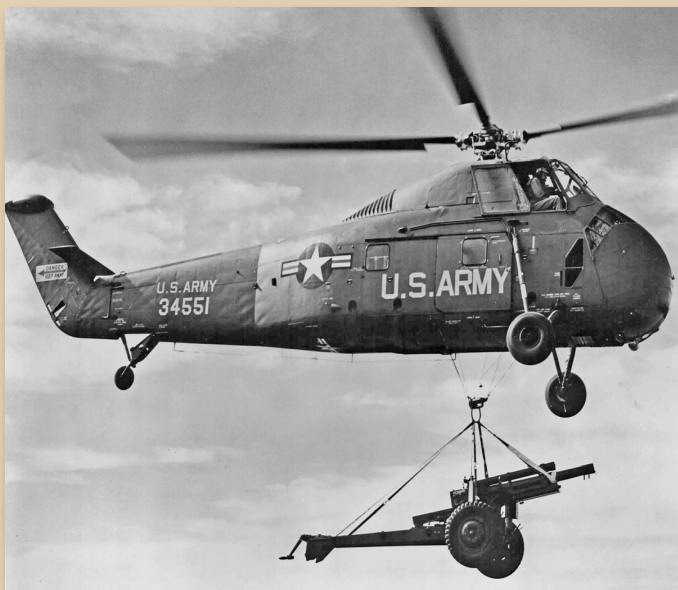
The S-58 (Army H-34 Choctaw) was the “light” cargo helicopter used to develop early airmobile concepts.
