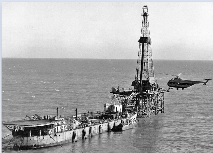
The piston-engined S-55 was the first transport category helicopter in offshore oil service, flying workers to rigs in the Gulf of Mexico in 1954.
