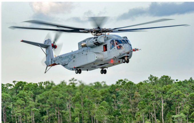
The S-95 or Marine Corps CH-53K King Stallion designed to replace the CH-53E entered development flight test in October 2015.
