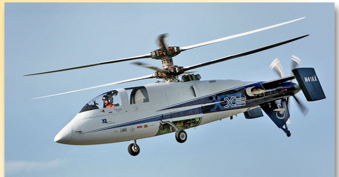
The Sikorsky-funded S-94 or X2 technology demonstrator integrated the advancing blade concept with structural, propulsion, and flight control advances.
