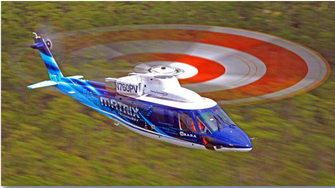
The S-76 Sikorsky Autonomy Research Aircraft was the first company-funded testbed for autonomous flight controls.
