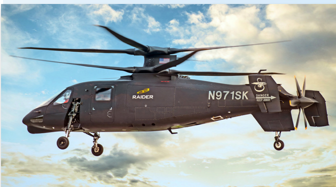
The S-92 Raider applied X2 technologies to a light tactical compound helicopter that exceeded 200 kt in October 2018.
