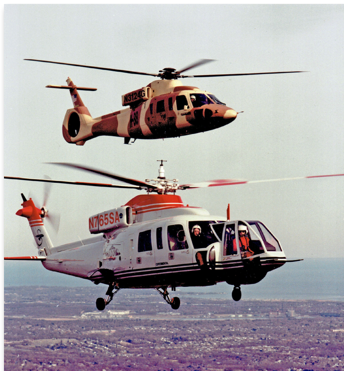
Sikorsky used the S-76 as the basis of its SHADOW flight control and FANTAIL shrouded tail rotor technology testbeds for the LHX program.
