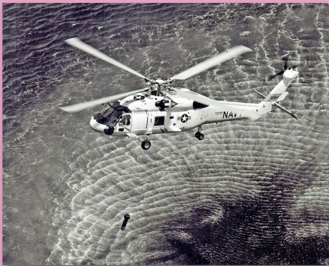
Sikorsky was prime contractor for the US Navy sonar-dipping SH-60F CV Helo.
