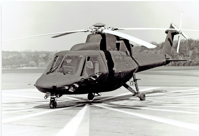
The S-75 built for the Advanced Composite Airframe Program proved the advantages of fiber-reinforced composites and began the transition to digital design.
