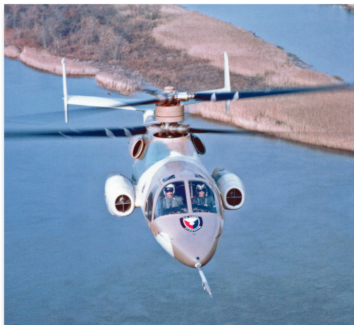
The S-69 Advancing Blade Concept tested compound helicopter technology for today's Defiant and Raider.
