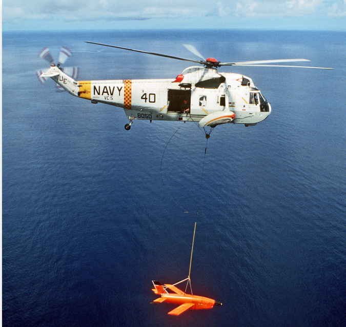
The Navy has long used helicopters like this SH-3G (S-61) to recover target drones, but Medium Range UAV plans included MARS to avoid saltwater infiltration and lengthy cleanup between missions. (Department of Defense)
