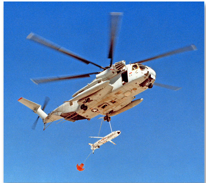
Three Air Force CH-53Bs (S-65s) were modified with MARS to support Air Launched Cruise Missile testing and drone experiments on the Utah Test Range. (National Archives)
