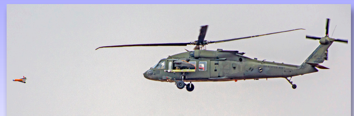
An Army MH-60M (S-70) launched Air Launched Effects (unmanned air vehicles) recovered by the unmanned Flying Launch And Recovery System during Project Convergence trials at Yuma. (US Army)
