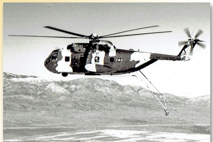
Air Force CH-3Cs (S-61Rs) with MARS rigs went to Southeast Asia in 1966 and remained essential to reconnaissance drone operations over North Vietnam. (Sikorsky Archives)
