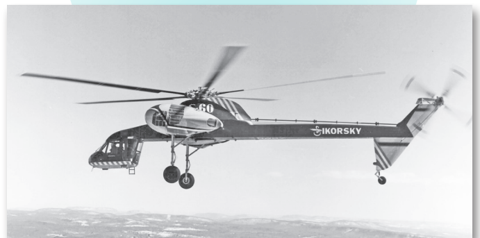
The S-60 flying crane demonstrator first flew on March 25, 1959 with the rotor system and engines of the S-56 and provided the basis for the turbine-engined S-64 Skycrane.
