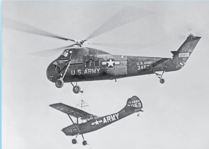
In 1953, the S-58 (CH-34 Choctaw) gave the US Army a transport helicopter powerful enough to recover downed aircraft. The S-58 went on to global military and commercial service and international production.
