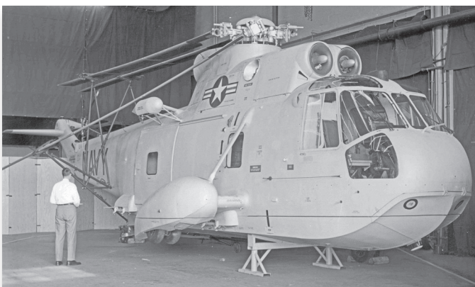
The S-61 mock-up at Bridgeport showed the twin turbine engines, boat hull, and five-bladed rotor system that would distinguish the record-breaking HSS-2 Sea King.
