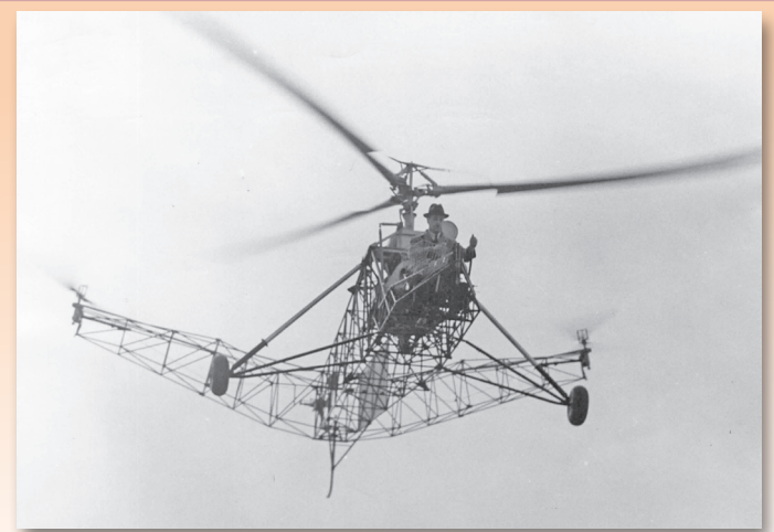
Igor Sikorsky flew his first public helicopter demonstration in 1940 with the VS-300 configured with three tail rotors.
