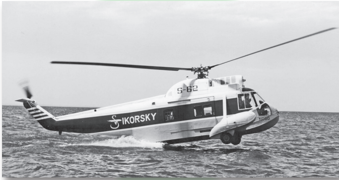
The turbine-engined, boat-hulled S-62 demonstrated water operations in 1958 and went on to production for the Coast Guard as the HH-52A Seaguard.
