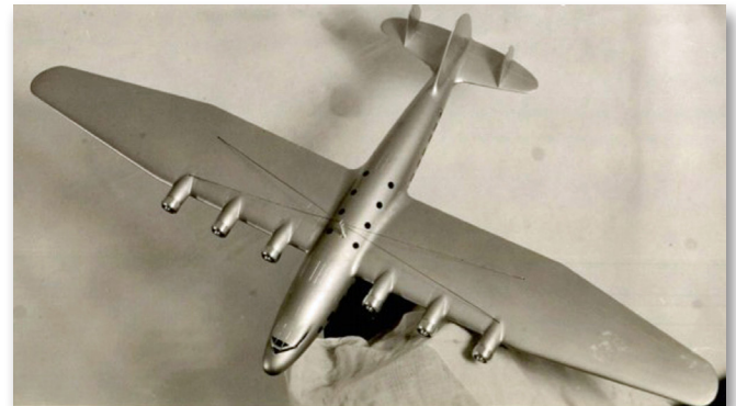
④. A 1938 design concept, designated as the S-45, would carry 100 passengers nonstop from New York to London. The project was terminated.
