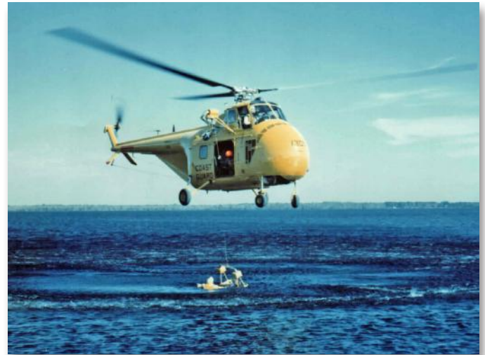
The S-55 (HO4S-1) gave the Coast Guard a helicopter with night/instrument flight capability. (Igor I. Sikorsky Historical Archives)
