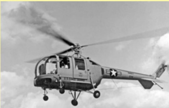
The S-52 (HO5S-1G) in the Coast Guard was the first Sikorsky helicopter with all-metal rotor blades but had only a short operational career
