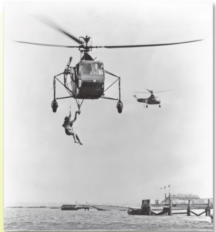
An S-47 (HNS-1) from Brooklyn flew hoist rescue demonstrations in Jamaica Bay. (Igor I. Sikorsky Historical Archives)
