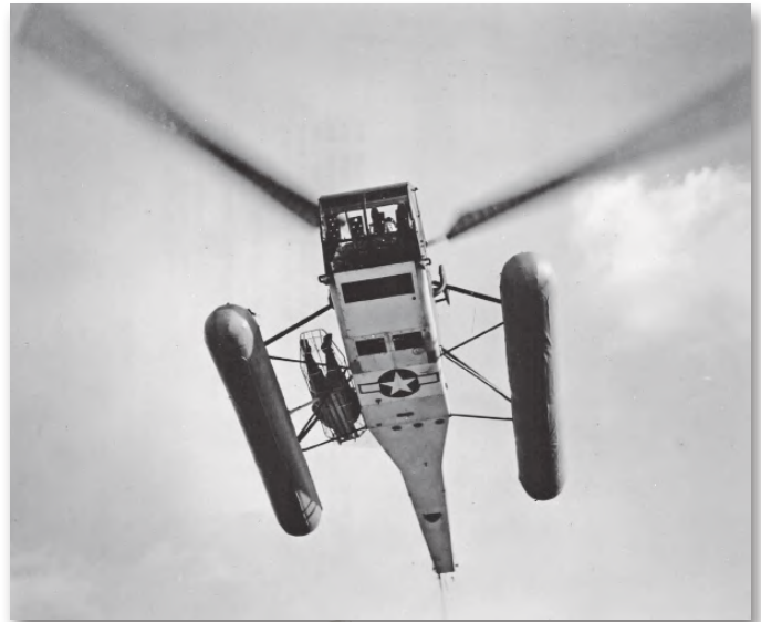
The Coast Guard S-47 (HNS-1) at Coast Guard Air Station Brooklyn was used to develop helicopter rescue hoists in 1944. (Igor I. Sikorsky Historical Archives)
