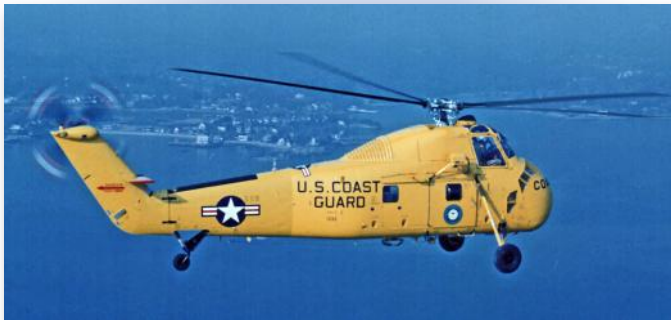
The S-58 (HUS-1G) introduced hands-off night hover capability but was used only briefly by the Coast Guard. (Igor I. Sikorsky Historical Archives)
