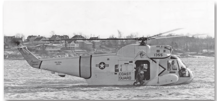
The turbine-powered S-62 or HH-52A Seaguard had a boat hull and fold-down recovery platform for water rescues. (Igor I. Sikorsky Historical Archives)
