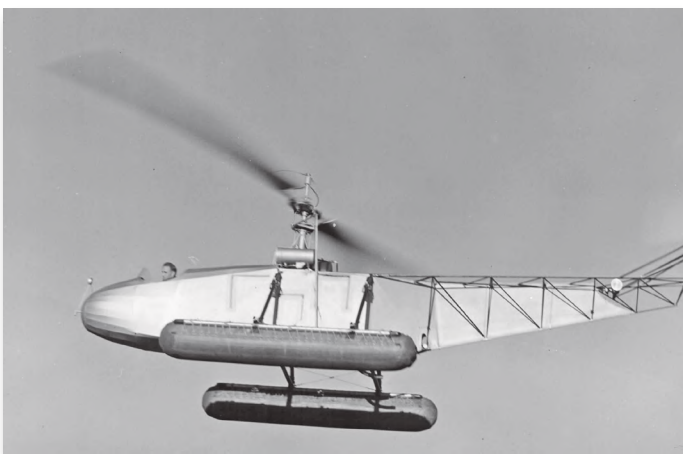
The VS-300 flew successfully with a two-bladed main rotor, albeit with higher vibration levels.
