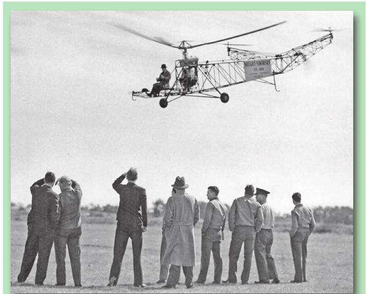
The VS-300 used two horizontal tail rotors on outriggers to provide pitch and roll control.
