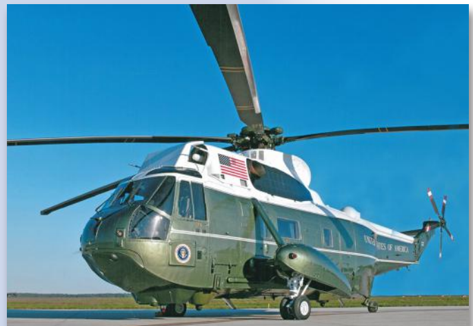
The VH-3D was upgraded with Carson composite main rotor blades. (Carson Helicopters)
