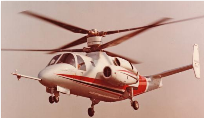
The XH-59 Advancing Blade Concept advanced Sikorsky's vision of high-speed helicopters. (Sikorsky Archives)
