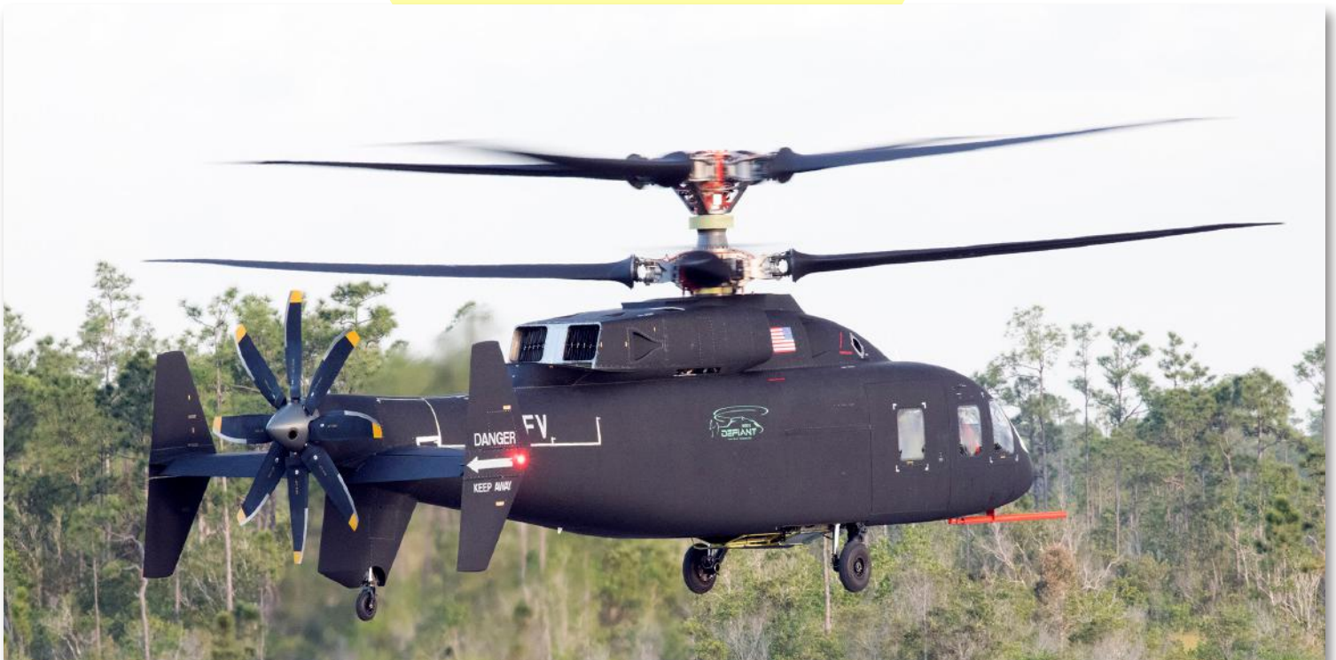
The SB>1 Defiant is the Sikorsky-Boeing Joint-service Multi-Role technology demonstrator (JMR-TD) with high-speed compound helicopter technologies for military Future Vertical Lift and commercial markets. (Sikorsky Boeing)
