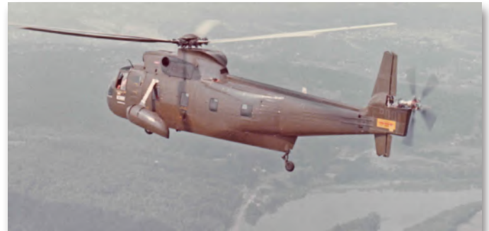
The Rotoprop was installed on a S-61 testbed and could pivot to the left for anti-torque control or aft for high speed thrust. (Sikorsky Archives)
