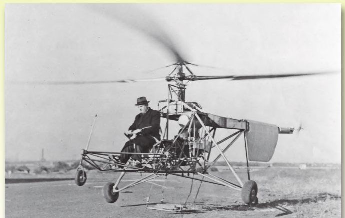
The VS-300 demonstrated Igor Sikorsky’s solution to the “helicopter problem” with controllable vertical flight. (Sikorsky Archives)
