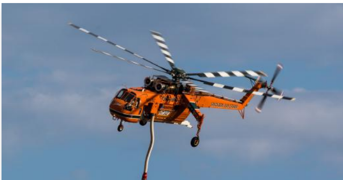
The S-64 Skycrane (Army CH-54 Tarhe) proved the value of crane helicopters. This modernized Erickson Airplane is configured to fight forest fires. (Erickson Inc.)
