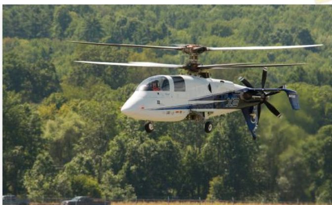
The Sikorsky X2 demonstrator integrated multiple technologies to make the high-speed compound helicopter practical. (Sikorsky Archives)
