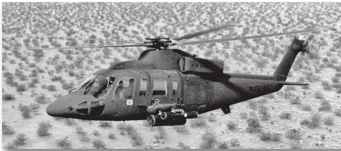
The AUH-76B became the H-76 Eagle with Pitch Compensated Armament Pylon, shown here with mixed rocket pods. (Sikorsky Archives)
