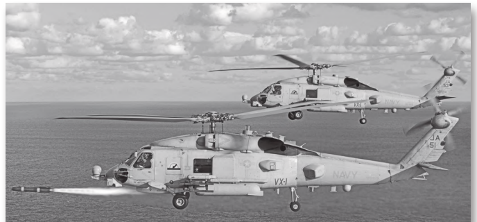
The latest MH-60R can use its electro-optical sensors to target laser-designated Hellfire missiles. (Sikorsky Archives)
