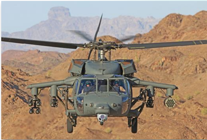
The S-70M Black Hawk today carries a mix of qualified weapons on its External Stores Support System. (Sikorsky Archives)
