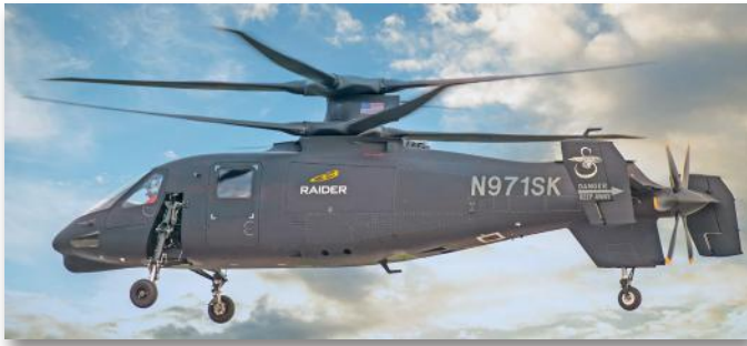
The S-97 Raider compound helicopter is sized for the scout-attack mission. (Sikorsky Archives)
