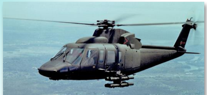
The AH-76A had a cabin floor beam to carry TOW missiles (shown here), rockets, or guns. (Sikorsky Archives)
