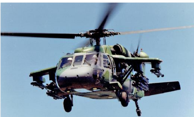
An international Black Hawk demonstrator carries Hellfire and Stinger missiles on its ESSS. (Sikorsky Archives)
