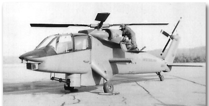
The S-71 was smaller but more powerful than the S-67 and designed to meet Advanced Attack Helicopter Requirements. (Sikorsky Archives)
