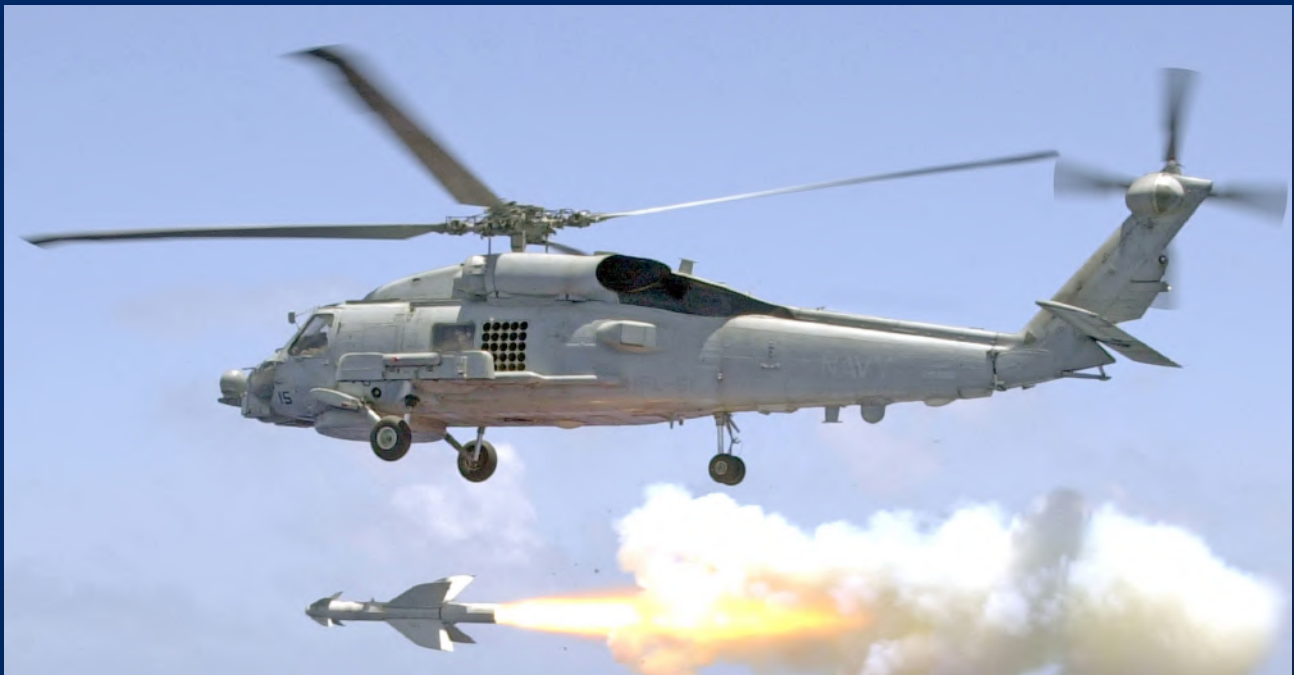
The International Naval Hawk integrates radar with Electronic Support Measures to target Penguin anti-ship missiles. (Sikorsky Archives)
