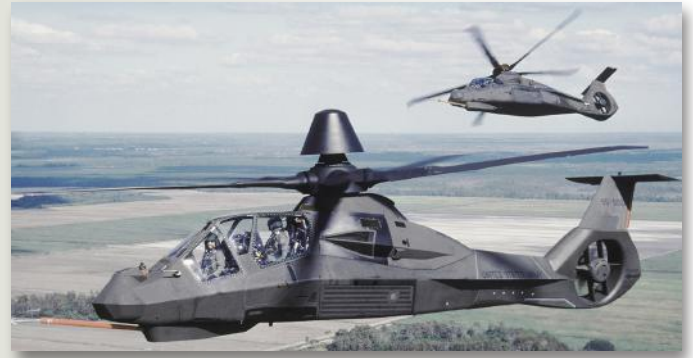
The RAH-66 Comanche packed weapons in a Low Observable helicopter with a highly integrated avionics architecture. (Sikorsky Archives)
