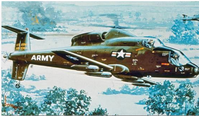
The S-66 compound helicopter used a swiveling rotoprop to attain its high speeds. (Sikorsky Archives)
