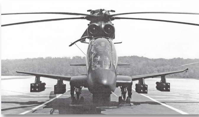
The S-67 Blackhawk attempted to answer the AAFSS requirements after the Cheyenne cancellation. (Sikorsky Archives)
