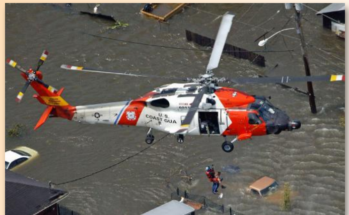
The Coast Guard HH-60J Jayhawk has been updated to the digital MH-60T. (Sikorsky)
