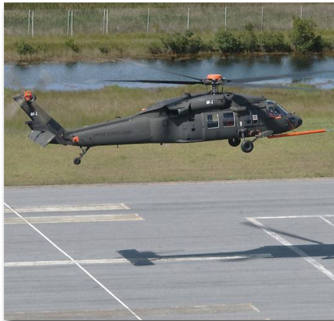
The first UH-60M was a conversion of an analog Black Hawk. (Sikorsky)
