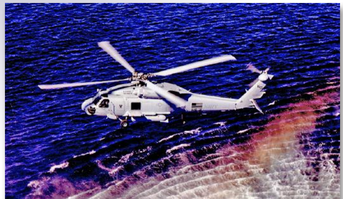
The S-70B-4 or SH-60F CV Helo was the carrier-based ASW helicopter of the U.S. Navy. (Sikorsky)
