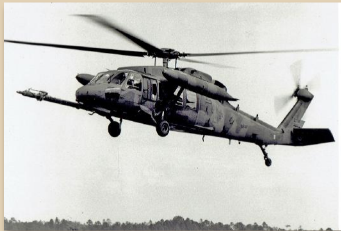
The Air Force HH-60D Night Hawk was to provide a Combat Search and Rescue helicopter. (Sikorsky)
