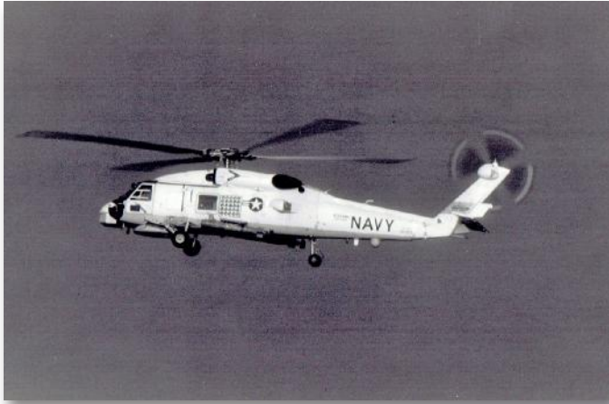
The SH-60B Seahawk gave the Navy its Light Airborne Multipurpose System. (U.S. Navy)
