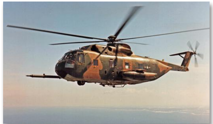
The S-61R/HH-3E Jolly Green Giant with air refueling capability extended rescue range in Southeast Asia. (Sikorsky Archives)
