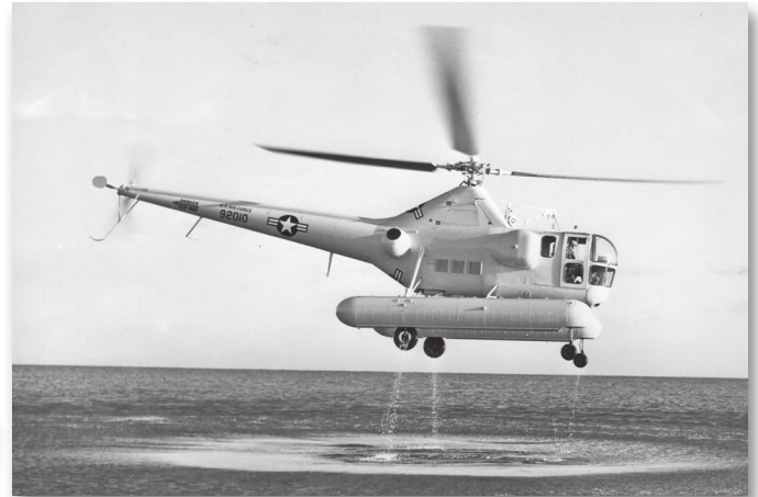
The S-51/H-5H with floats, hoist, and cabin litter provisions remained in Air Force service until 1962. (Sikorsky Archives)
