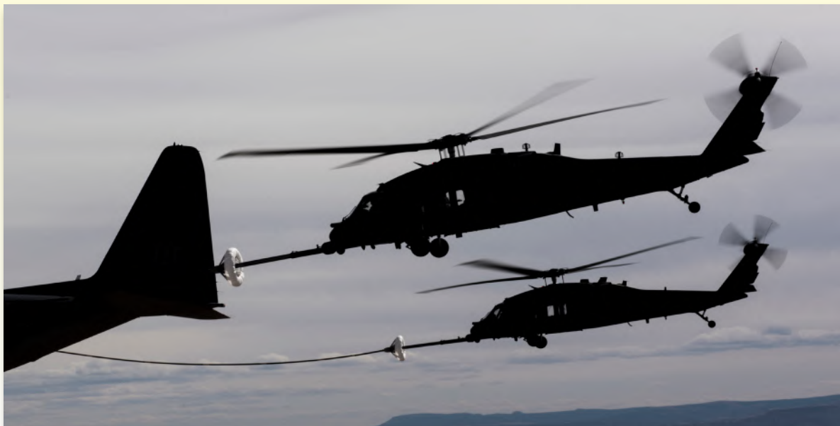
The Pave Hawk evolved from the BLACK HAWK with air refueling and rescue avionics. (U.S. Air Force)
