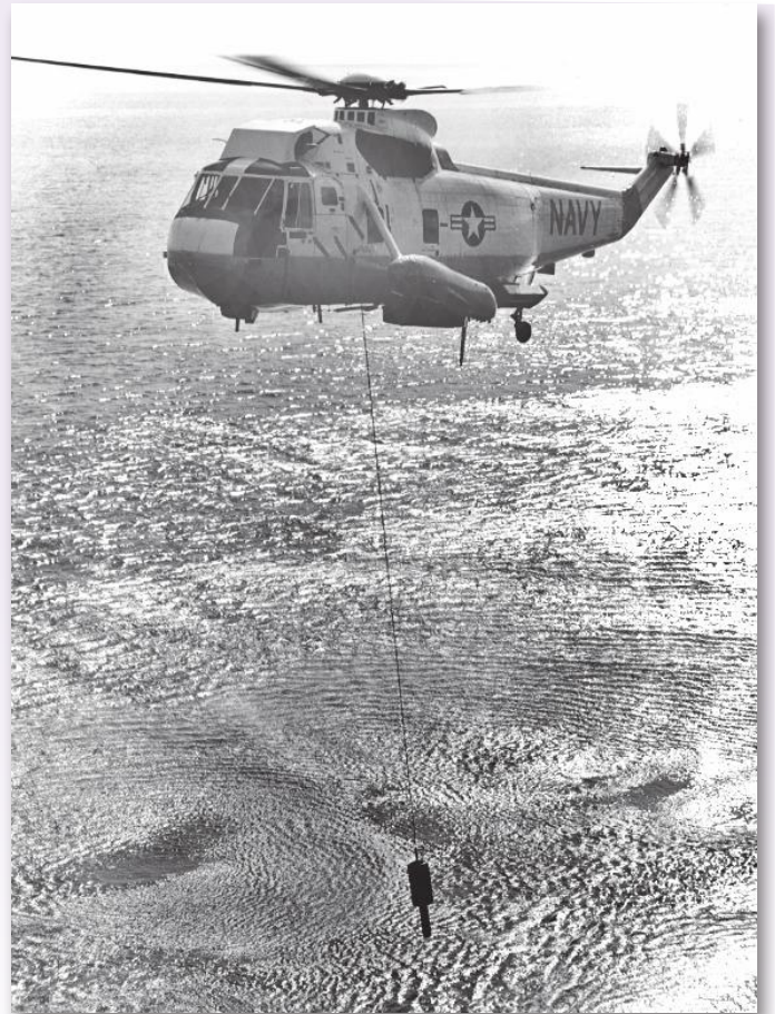
The SH-3H hunted with sonar, MAD, radar, and Electronic Support Measures. (Sikorsky Archives)
