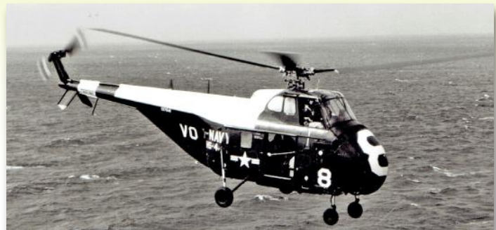
The S-55 (HO4S-3) could carry either dipping sonar or a torpedo and had to work in hunter-killer teams. (Sikorsky Archives)
