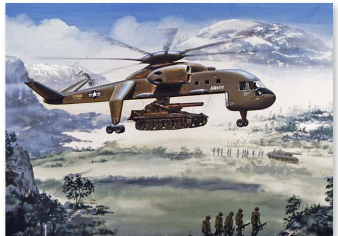
Large Crane Helicopter Using Dual Tail Rotors and V Tail
