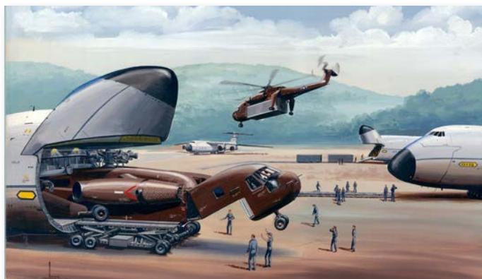
Folded S-64 Being Loaded in a C-5 Transport
