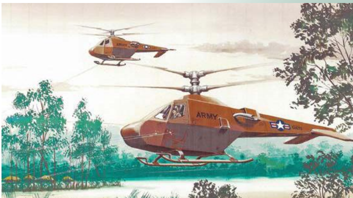
Advancing Blade Concept Helicopter with Steel Armored Plate Fuselage
