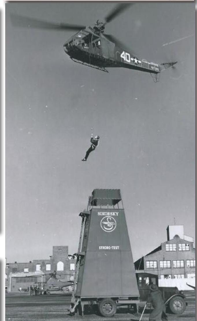
Sergei hoisted from a platform atop a movable stroboscopic tower at the Bridgeport Sikorsky Aircraft factory. The aircraft shown has skid landing gear which was not used in production.
