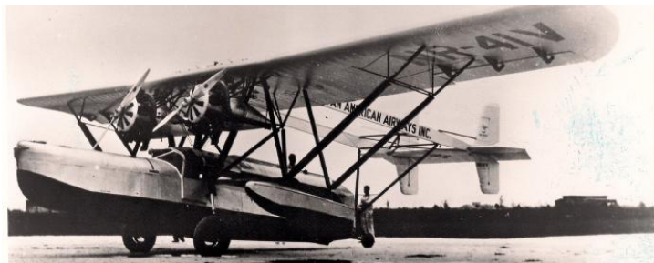
S-41 was a larger twin engine derivative of the S-38. Seven were built.
