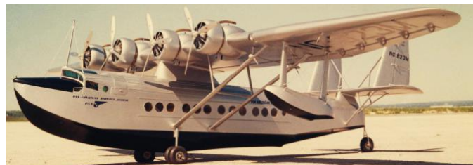
The four engine S-42 could carry 35 passengers and was the largest flying boat at the time. Ten were built.
