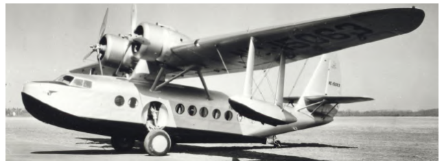
S-43 Baby Clipper was a twin engine amphibian that could carry 15 passengers. They were used in military and commercial service. 53 were built.
