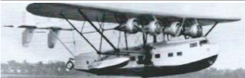
S-40 "The American Clipper" started as a four engine amphibian type aircraft. Three were built and in 1935, they were modified to flying boats when the landing gear was removed to save weight.
