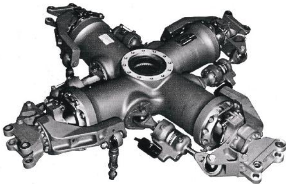
S-70 (H-60) elastomeric spindle assemblies installed in each main rotor hub arm of the one piece propeller hub
