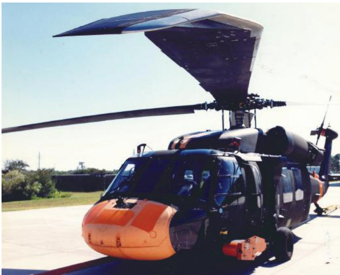
S-70 (UH-60M) High Performance Titanium Main Rotor Blade with adhebral shape tip developed in early 2000s. Prior blades had no adhebral tip shape. Current production blades have composite spars.
