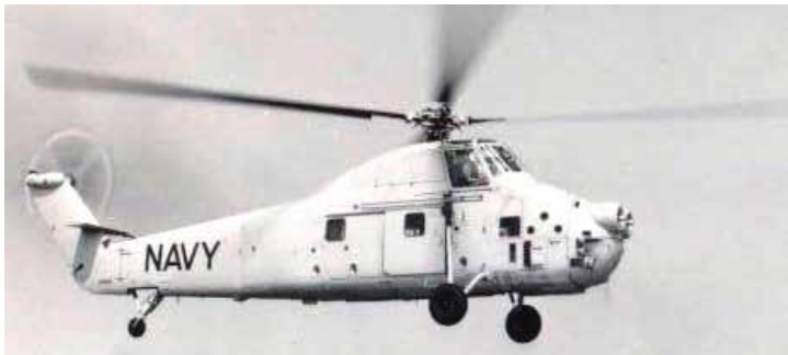
S-58 (SH-34) with two GE T-58 engines
