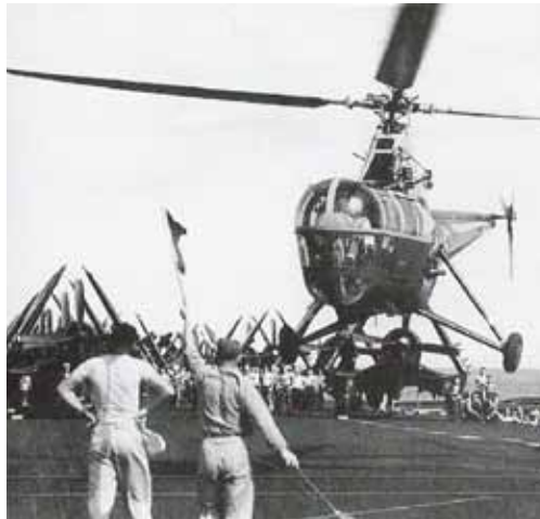
The Landing Signal Officer directs an S-51 (HO3S-1) Helicopter Landing On The FDR
