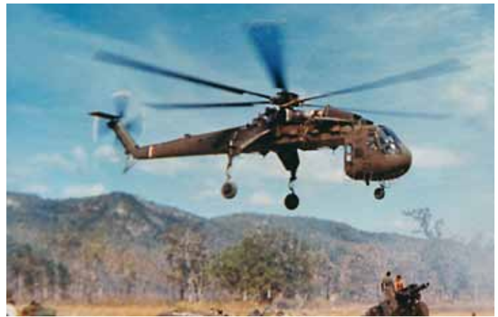
CH-54 is shown with Engine Air Particle Separators to extend engine life from 8 to beyond 600 hours Time Between Overhaul in abrasive environments
