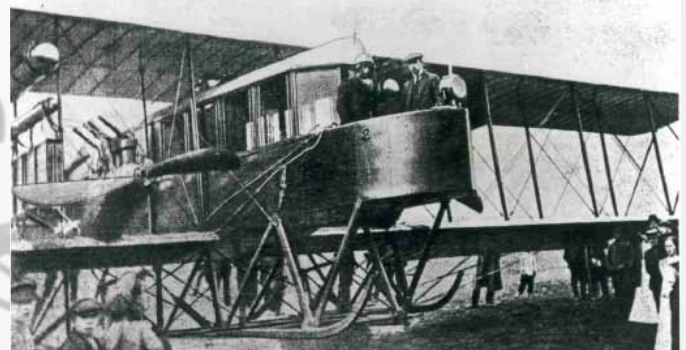
▲ S-21 first four engine aircraft in the world, with Igor Sikorsky in the open nose compartment
