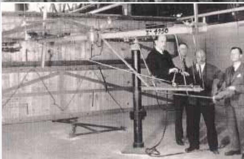
The first Helicopter rotor system flight control simulator with Igor Sikorsky at controls, and observers Michael Buivid, Boris Labensky and Michael Gluhareff
