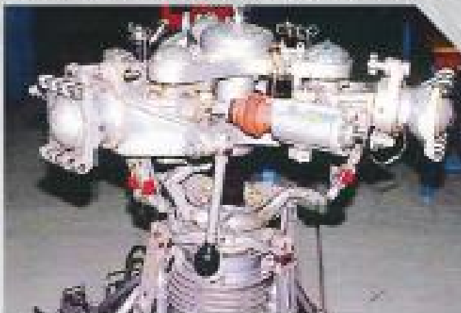
S-55 Main Rotor and Main Gearbox Assembly
