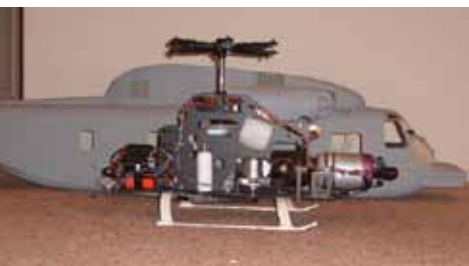
Main, Transmission, and Engine in position relative to fuselage
