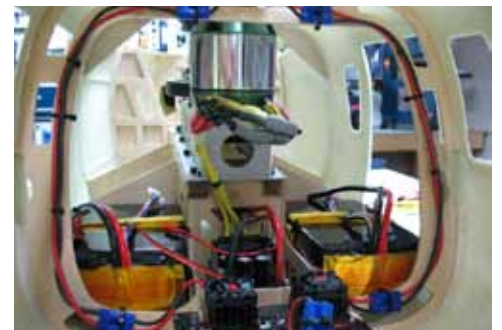
Electric Motor and Batteries in Cabin
