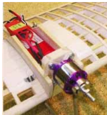
Typical of the four engine installations in the wing
