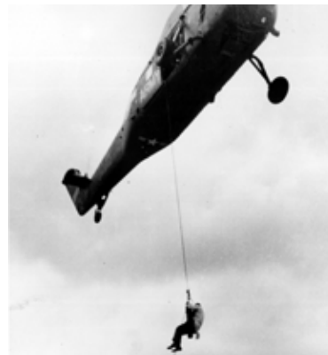
Sikorsky pilot Frank Yirrel performing a rescue with an Army S-58 helicopter using a rubber tire on a sling, due to lack of an aircraft rescue sling
