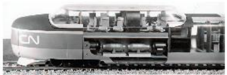
Figure 1-Power Dome Car Model
