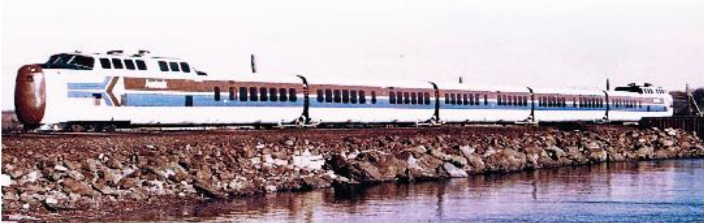
Amtrak TurboTrain showing Power Dome Cars at each end
