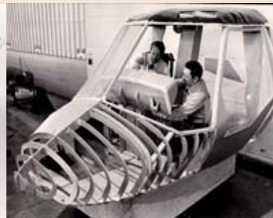
Joe Keogan and Bill Jennings building the S-76 cockpit mock-up
