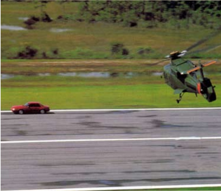
Fantail Aircraft Paced By Ground Vehicle During Sideward Flight Testing at WPB, FL
