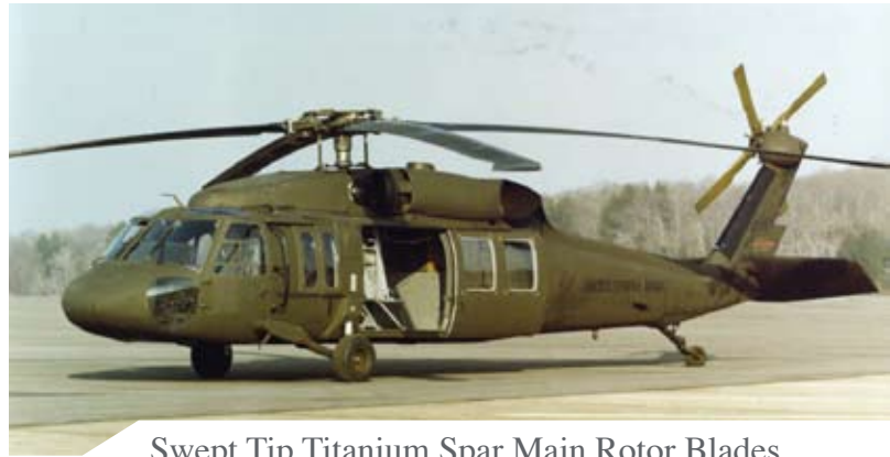
Swept Tip Titanium Spar Main Rotor Blades
