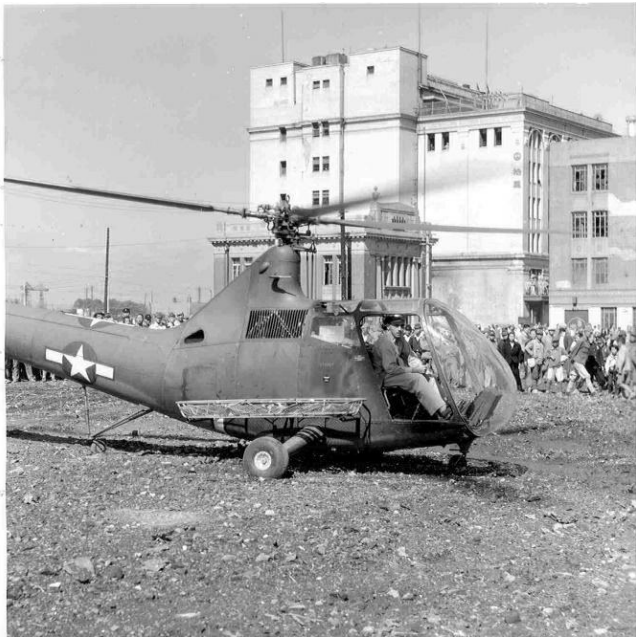
Figure 40: Lieutenant John Noll with side-mounted Stokes Litter during a Sikorsky R-6A helicopter demonstration
