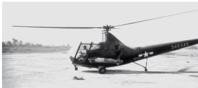
Figure 43: Flight Officer Edward Ciccolella delivering another wounded soldier using the side-mounted stretchers (Stokes Litters) on the R-6A Sikorsky helicopter
