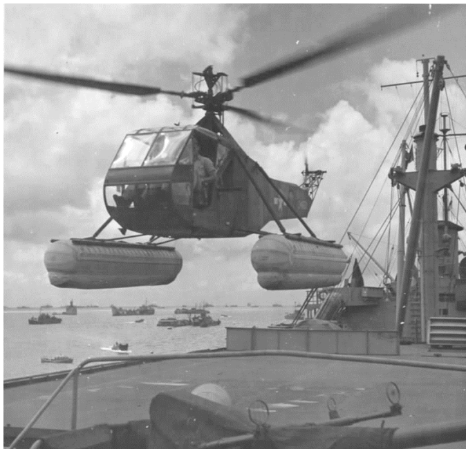
Figure 19: R-4B Sikorsky helicopter with floats landing on the Aircraft Repair Ship, Major General Roberts Olds (ARS-1)
